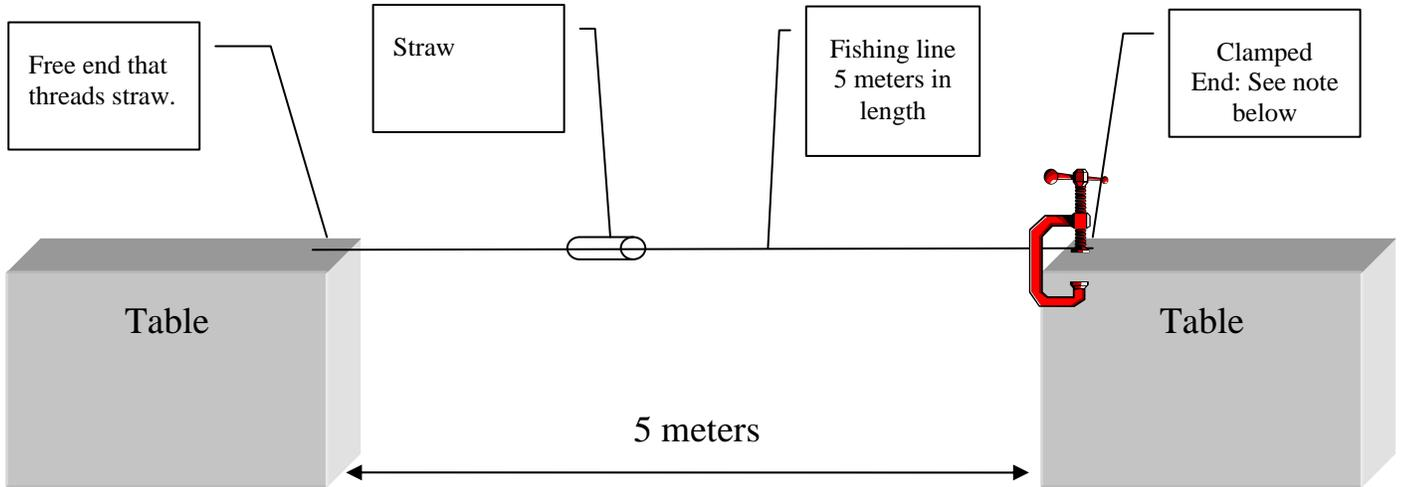
**For the clamped end:** the fishing line maybe difficult to clamp. To help, wrap a piece of duct or masking tape around the fishing line then clamp down on the taped end. See diagram below:
